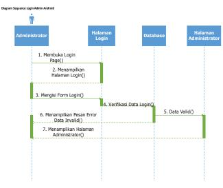
Fig. 4. Sequence Diagram of the Android Administrator Login
